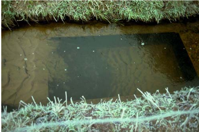
Fig. 1: Sediment trap in the Endeholz Ditch to quantify the load of fine sediments. The wooden box (Size: 2 m long, 1 m wide, 0.5 m deep) is open on the top. The sandy material which is mostly transported by rolling over the substrate, along with organic material is deposited in and caught by the box. The sand ripples which are seen in Fig. 1 on the left are typical of an unnaturally high sandy load and are more characteristic of a beach than the bottom of a natural heather creek.
